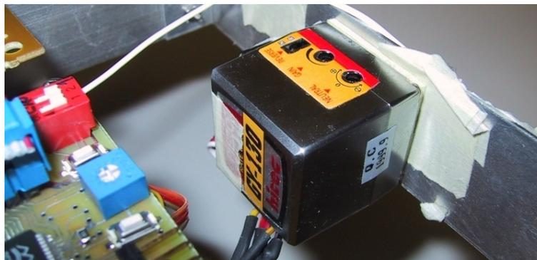
**Fig. 2.14 – One of the two gyros that equip the body**
