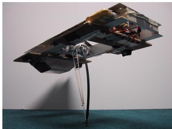
**Fig. 1.2 – The 3D Bow Leg Hopper**
