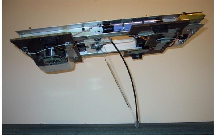
**Fig. 2.4 – Left: Raibert’s one-leg hopping robot from [wwwLegLab] - Right: the 3D Bow Leg Hopper**
